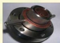
Broadband transmission of RF signals into cryogenic UHV Cavity. 50 Ohm Impedance Matched. Copper-alloy components sealed to alumina ceramic. UHV metal-sealed flange mount. Integrated liquid cooling.
